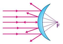
The bulging surface of the convex mirror reflects light outwards
